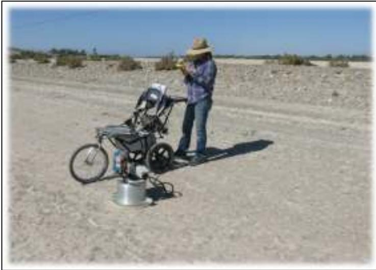
Portable In Situ Wind Erosion Lab
