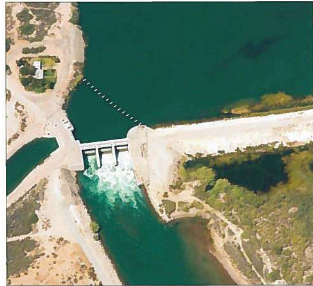
PALO VERDE DIVERSION DAM, right, serves Palo Verde Irrigation District. It was built during World War II, replacing a rock weir.
